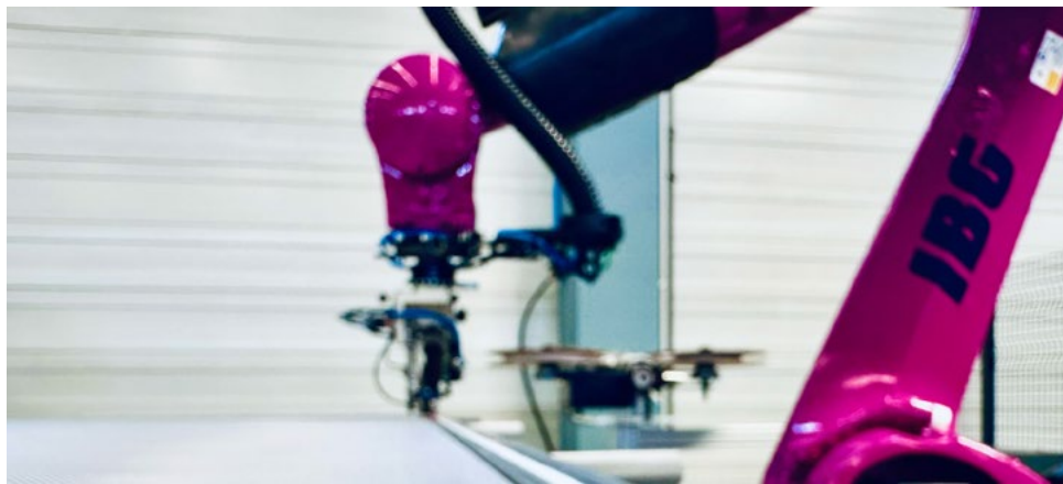
A robot in the "NCAlab" laboratory and test center performing the sealing of a half-shell.
