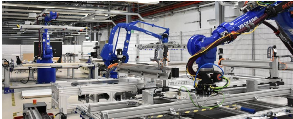
A test assembly system at TU Braunschweig designed for the automated assembly of AWE electrolysis cells, with an emphasis on process interlinking.
